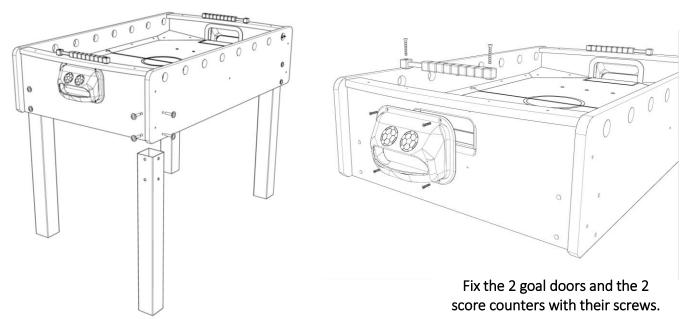
Assemble and fix all 4 legs with their metal flat and screw (8x45 ) by using the Allen spanner key (5)
