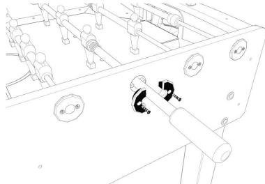
Fix the other side of the rod (handle side) with the 2 bushings; one from inside and one from outside by affixing all components with the use of the 2 screws.
